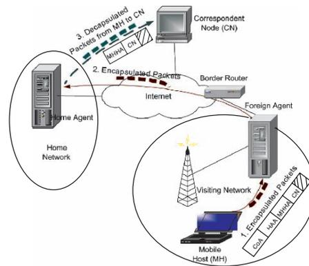
Figure 9: Interoperability between Mobile IP and Ingress Filtering.
