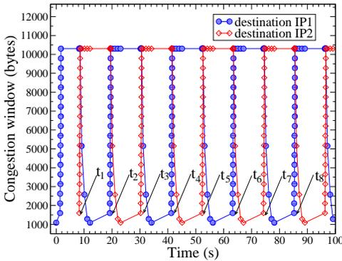
Fig. 4. CN's congestion window during one handover with no layer 2 setup latency.
