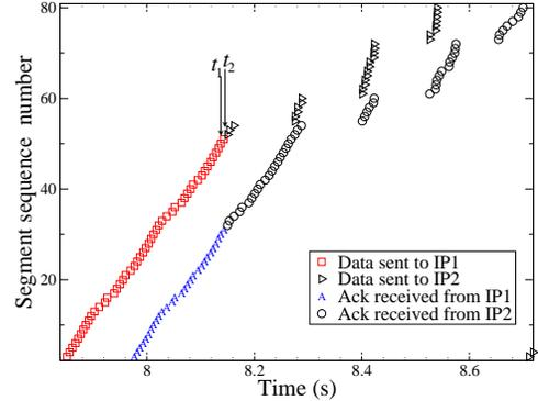
Fig. 5. Segment sequence of SIGMA during one handover with layer 2 setup latency of 200ms.
