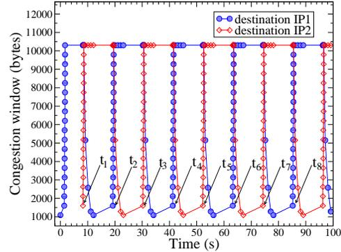
Fig. 6. CN's congestion window during one handover with layer 2 setup latency of 200ms.
