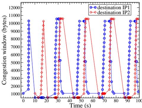
Fig. 8. CN's congestion window during one handover with layer 2 setup latency of 500ms.
