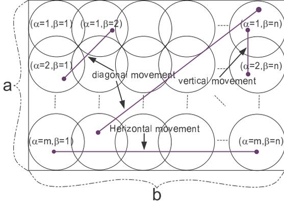
Fig. 4. Arrangement of subnets in a rectangular topology.
