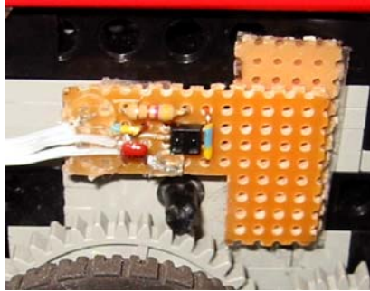
Figure 2 Custom wheel encoder
