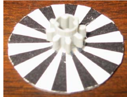
Figure 3 12 stripe encoder wheel
