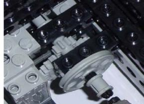
wheel. This two-gear system would spin the encoder at three times the rpm of the driven wheel.
