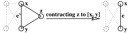
Fig. 5. If z is a degree-2 node which makes a triangle with link [x, y] , we can contract node z to link [x, y] . When we perform this contraction operation, the subgraph G(x, y) is expanded to include also the union of G(x, z) and G(z, y) . Therefore the subgraph represented by link e is the union of G(e') , G(x, z) , and G(z, y) . Also, the link attributes of e is computed from the link attributes of e' , (x, z) and (z, y) in O(1) time.
