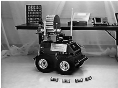
Fig. 2. A team for distributed exploratory missions - a ranger (center) with four scouts (foreground)
