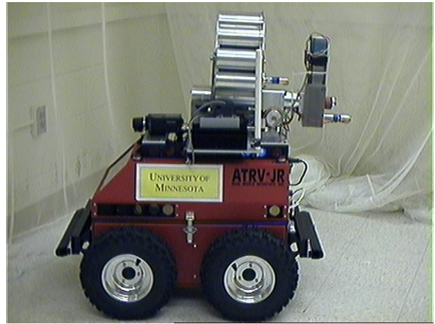
Figure 2: A ranger robot with scout launcher.
