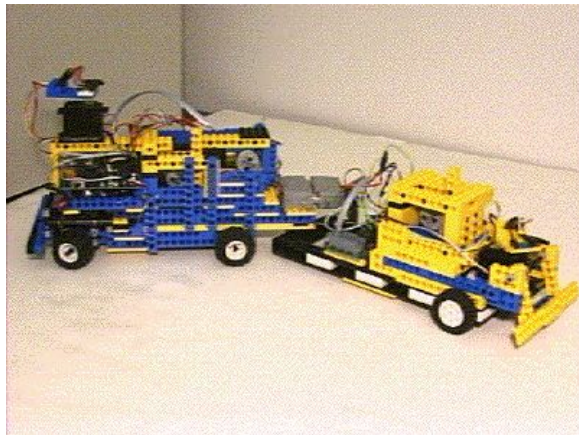
Figure 7: The Self-Positioning Trailer-Backing Mini-robot
