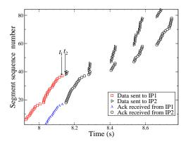
Fig. 3. Segment sequence of SIGMA during one handover with no layer 2 setup latency.
