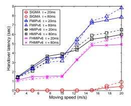
Fig. 10. Impact of moving speed and layer 2 beacons
