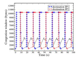
Fig. 4. CN's congestion window during one handover with no layer 2 setup latency.
