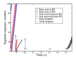
Fig. 7. Segment sequence of SIGMA during one handover with layer 2 setup latency of 500ms.
