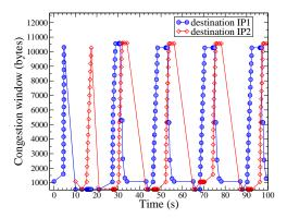
Fig. 8. CN's congestion window during one handover with layer 2 setup latency of 500ms.
