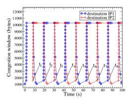
Fig. 6. CN's congestion window during one handover with layer 2 setup latency of 200ms.
