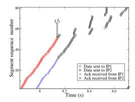
Fig. 5. Segment sequence of SIGMA during one handover with layer 2 setup latency of 200ms.
