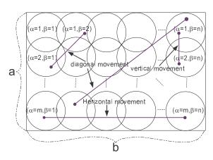
Fig. 4. Arrangement of subnets in a rectangular topology.
